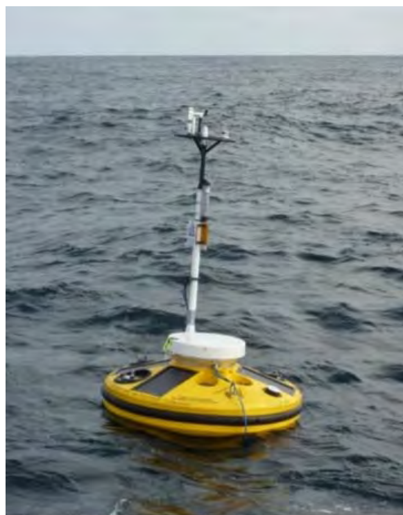
SEAWATCH Wavescan buoy with met mast
